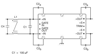
$C1 = 100 \,\mu\text{F}$   $C2_a - C2_b = 4,700 \,\text{pF}$  $C3_a - C3_b = 0.01 \,\mu\text{F}$
